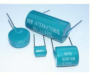
This sintering process produces a Ceramic Carbon Resistor which is 100% active material and therefore of minimum size. The H.V. Resistors for Compact Circuitry range feature radial lead terminations and a high quality epoxy resin coating to improve both dielectric withstand and mechanical robustness.
